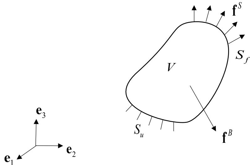
$$\text{PVW: } \int_V \tau_{ij} \delta \varepsilon_{ij} dV = \int_V f_i^B \delta u_i dV + \int_{S_f} f_i^S \delta u_i dS$$
