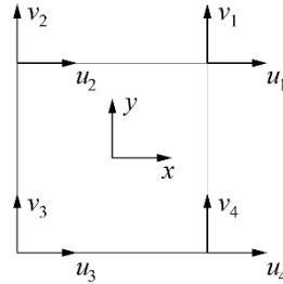
$$u = \underbrace{\frac{1}{4} \left(1 + \frac{x}{2}\right) \left(1 + \frac{2}{3}y\right)}_{h_1} u_1 + \underbrace{\frac{1}{4} \left(1 - \frac{x}{2}\right) \left(1 + \frac{2}{3}y\right)}_{h_2} u_2 + \underbrace{\frac{1}{4} \left(1 - \frac{x}{2}\right) \left(1 - \frac{2}{3}y\right)}_{h_3} u_3 + \underbrace{\frac{1}{4} \left(1 + \frac{x}{2}\right) \left(1 - \frac{2}{3}y\right)}_{h_4} u_4$$
